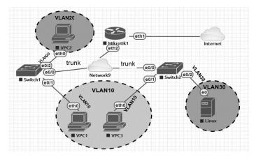
Fig. 2. Network topology with VLAN
